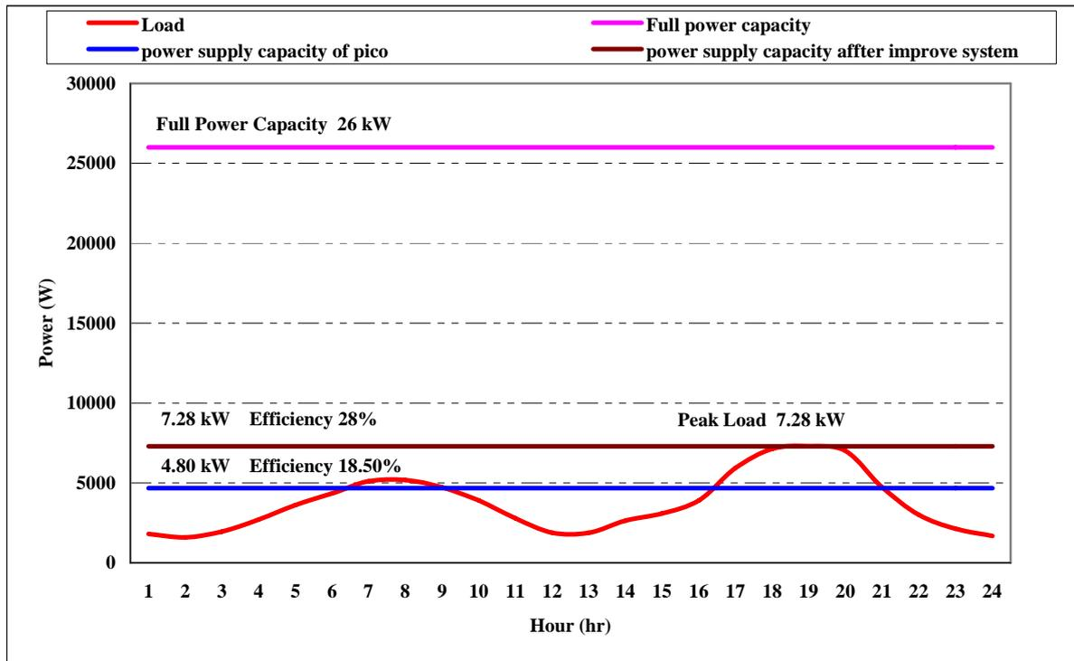
Fig. 7 Load Profile after improve the Efficiency Demand peak load 7.28 kW Power Supply Capacity 7.28 kW Out put Supply Efficiency 28 % Number of family 50 Household Load demand per family 145 W
